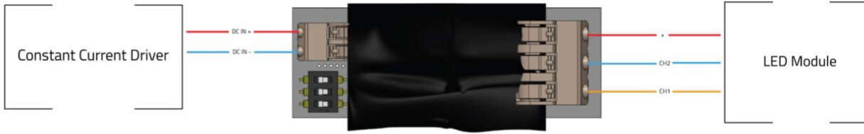
Figure 2 - APT-CC-VFW Adjustable fixed white configuration
