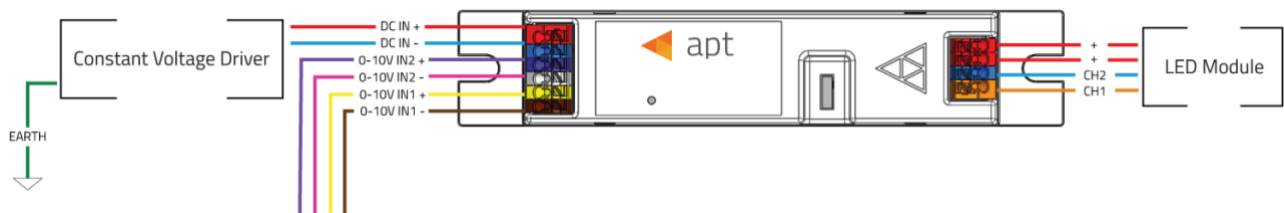
Figure 6 - APT-CV2-VD-LN Dual 0-10V Dimmer Configuration
