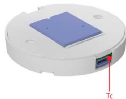
Figure 1: Tc point on ORB controller, micro USB connector shield
