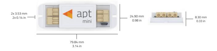
Figure 1 – Mechanical Drawing
