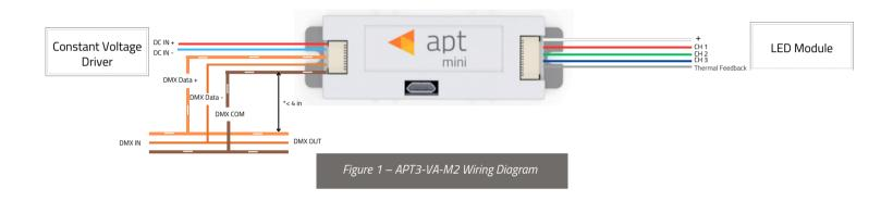
\*If no DMX splitter or amplifier is used, splitting between DMX IN/OUT should be done within 4 inches of the APT controller input connector to prevent line reflectance
