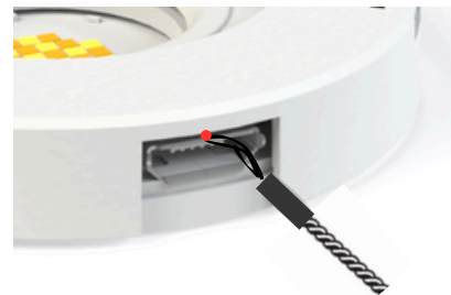
Fig. 3 - To measure Tc, insert thermal probe between micro-USB and top encasement as shown
