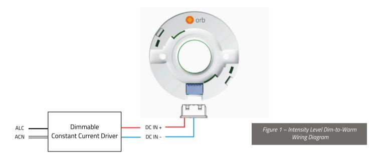
Constant current driver intensity control could be 0-10V or phase dimming. Driver compatibility testing is required.
