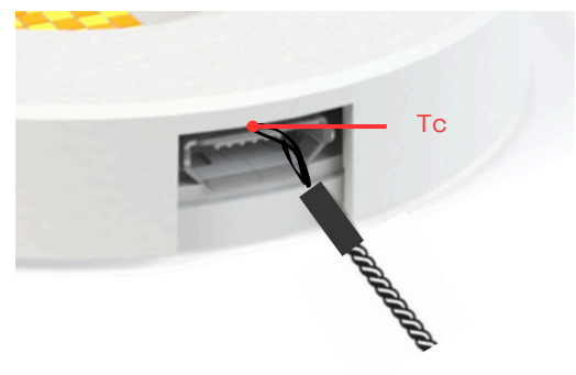
Figure 1 - Tc is measured on the metal sleeve of the micro-USB programming port. To measure Tc, insert thermal probe between micro-USB and top encasement of the ORB controller as shown.
