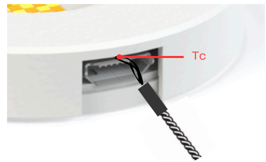
Figure 1 – Tc is measured on the metal sleeve of the micro-USB programming port. To measure Tc, insert thermal probe between micro-USB and top encasement of the ORB controller as shown.
