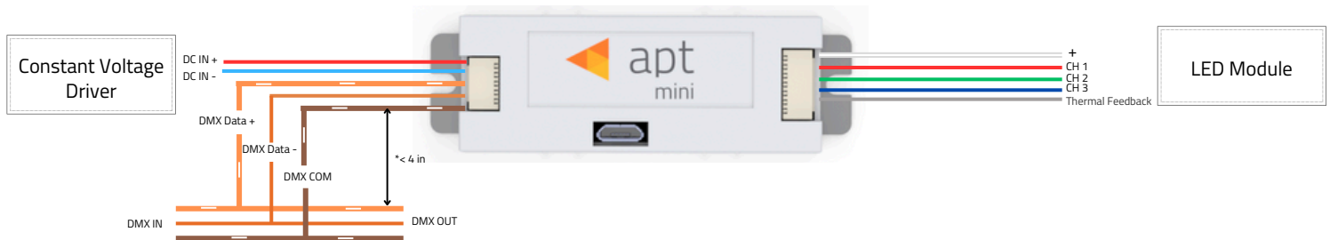
Figure 2 – APT3-VA-M2 Wiring Diagram
