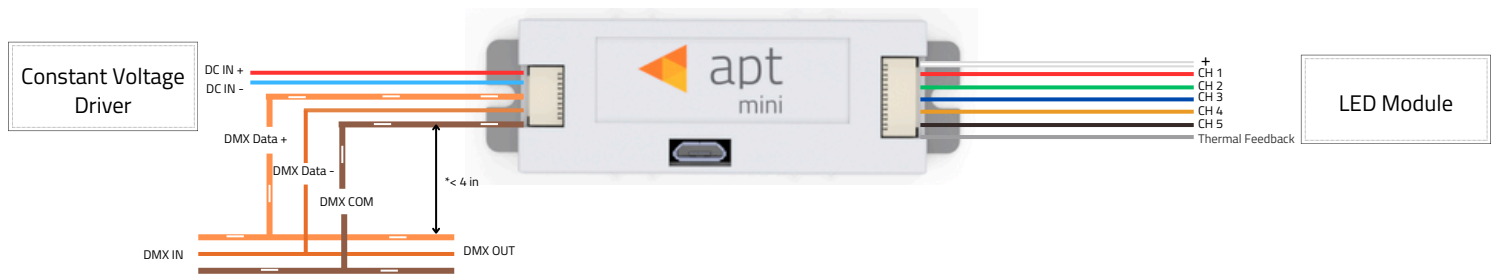
Figure 3 – APT5-VA-M2 Wiring Diagram
