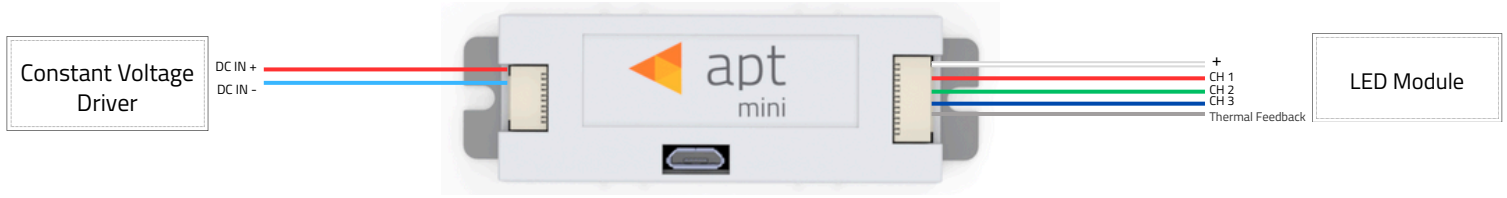
Figure 9 – APT3-VWC-M2 Wiring Diagram
