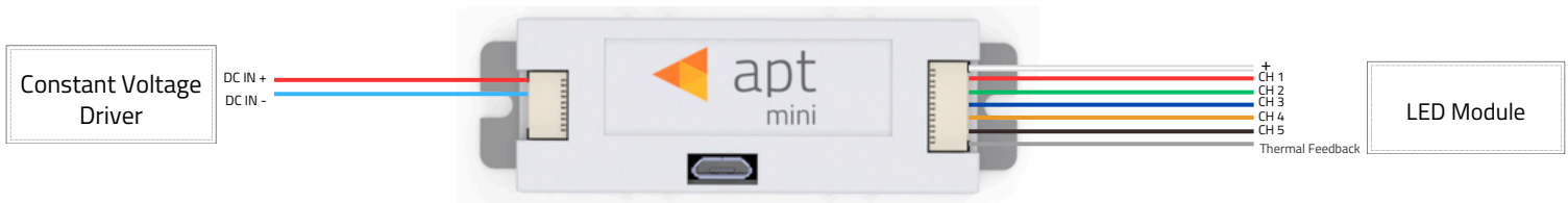
Figure 10 – APT5-VWC-M2 Wiring Diagram
